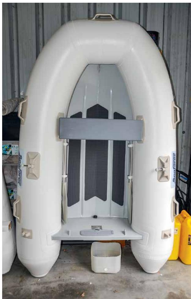
In addition to manufacturing its own RIBs the company also manufactures tubes for a range of other RIB builders, including Auckland’s Smuggler Marine. Seafarer also has a division specialising in repairs to all brands of RIBs – with tubes constructed in PVC, polyurethane and Hypalon.
